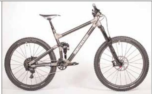
**The titanium lugs for Robot Bike Co.'s bespoke MTB bike frame were produced using Renishaw's selective laser melting process, an additive manufacturing technology that can build components directly from computer-aided design geometry using fine metal powders** © Renishaw/Robot Bike Co.
