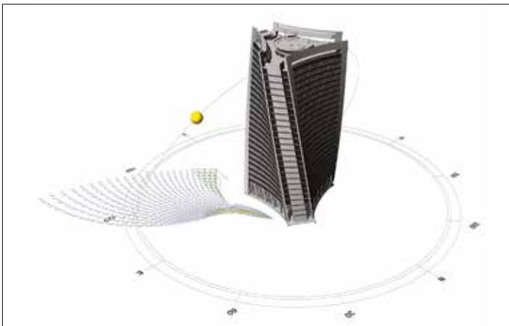
Analysis of the concentrated solar reflection from the curved glass facades of the PwC Tower © Arup
