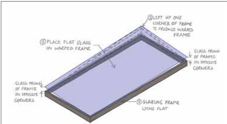
Each of the facade panels is warped to accommodate the twist, but a glazing sub-frame within the panel allows the glass to be flat and sit in one plane. All of the geometrical abnormalities were cleverly hidden within the depth of the frame © Arup
