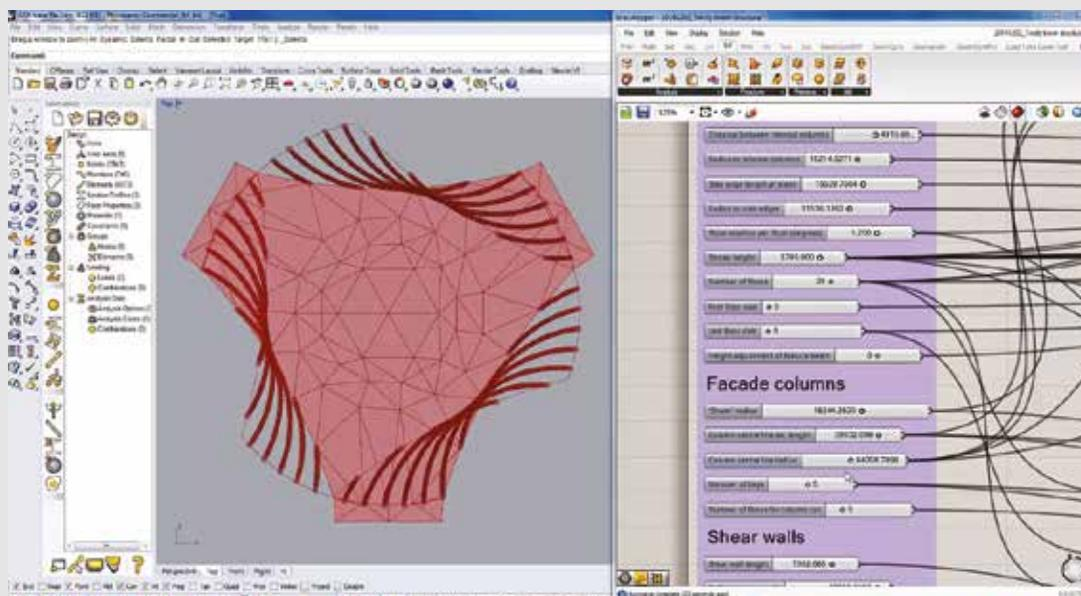
Parametric modelling is the modelling of a structure in n-dimensional space, where certain chosen parameters of the structure are variable. This allows the team to explore the impact of changing any of the input parameters on the design and cost of the structure, simply by moving a 'slider' on the screen © Arup
