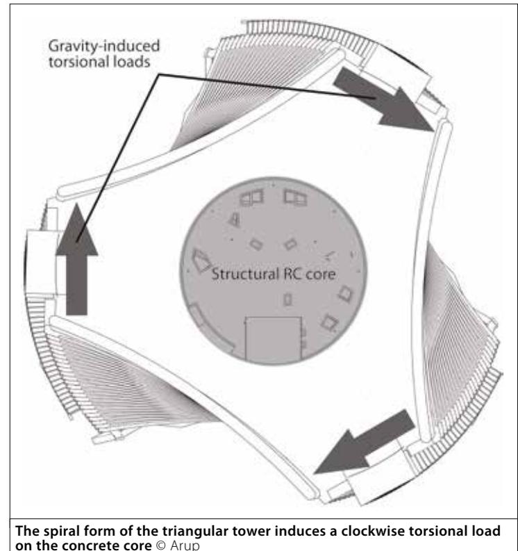
structure, in effect, slopes away from or towards the centre, and consequently generates no torsion. Unfortunately, this idea resulted in an irregular pattern of columns that detracted from the building’s spiralling form and did not fit with the aesthetics of the design.
