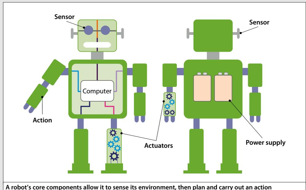
A robot's core components allow it to sense its environment, then plan and carry out an action
