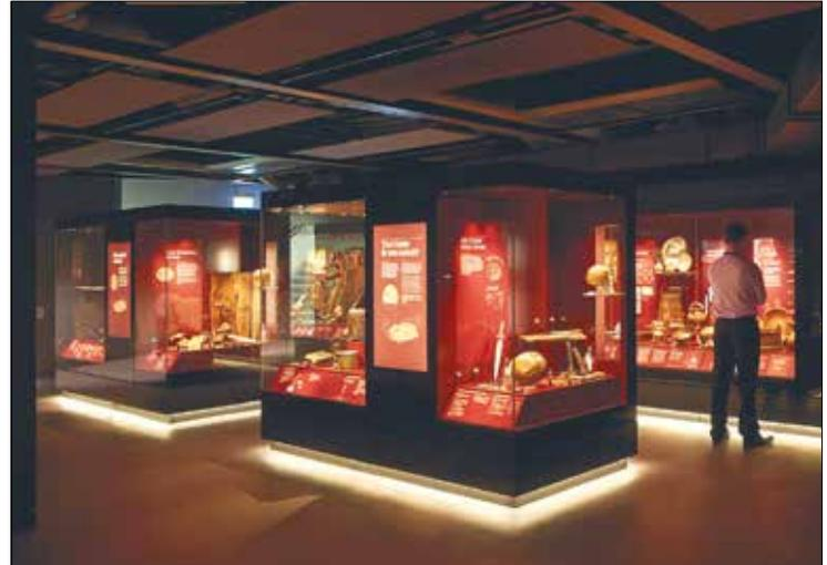
Museum display units often have a system of humidity control within the cases. The *Mary Rose* Museum has a micro-air-conditioning system for its display cases, each independent of the others, which are in turn connected to the chilled water system. The museum staff set the cases to 55% humidity and 19°C, which is typical for storing organic artefacts © Mary Rose Trust
