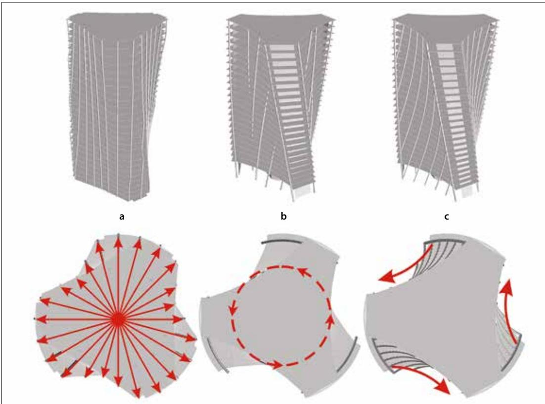
Plan and isometric sketch of each of the three alternative schemes for columns: (a) radially sloping columns; (b) internal spiral columns; (c) sloping facade columns © Arup
