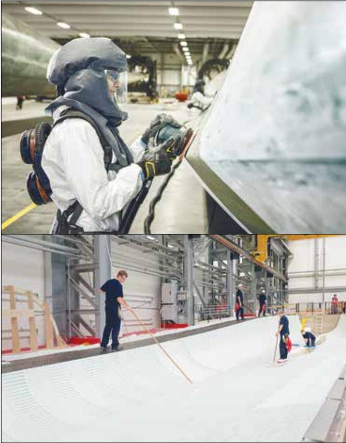
**Siemens makes 75-metre-long rotor blades at its new Green Port Hull factory. These blades, for 7 and 8 megawatt wind turbines, are individually made from fibreglass-reinforced epoxy. More recently, Siemens has introduced hybrid carbon blades. Different blade materials make it possible to tailor wind turbines for different locations, onshore and offshore and in areas with different wind conditions** © Siemens
