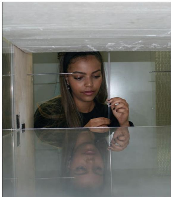
Abigail sets up an experiment by placing a total pressure pitot into its holder in her experimental rig
