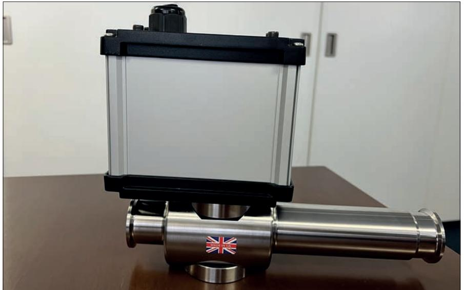
The sensor instrument mounted on a flow-through pipe. These pipes are used throughout the plant to transport liquids between tanks, from tanks to mixers, and eventually to the bottling unit © Phil Marsden
