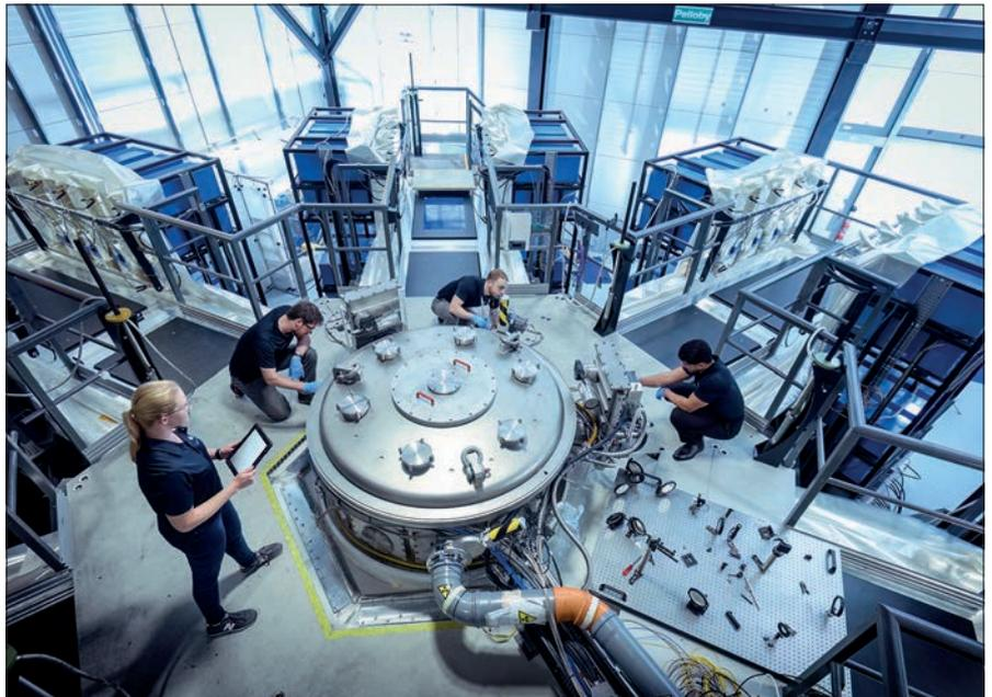
**‘Machine 3’, built in 18 months at a cost of £3.6 million, stores electrical energy in banks of capacitors. It uses electromagnetic forces to launch projectiles at the hypervelocity speed needed to test fusion targets. The projectiles hit the amplifier at 20 km/second. The company describes this as “one of the largest pulsed power facilities in the world and the largest in Europe”. It is also the only one built specifically for fusion research © First Light Fusion**
