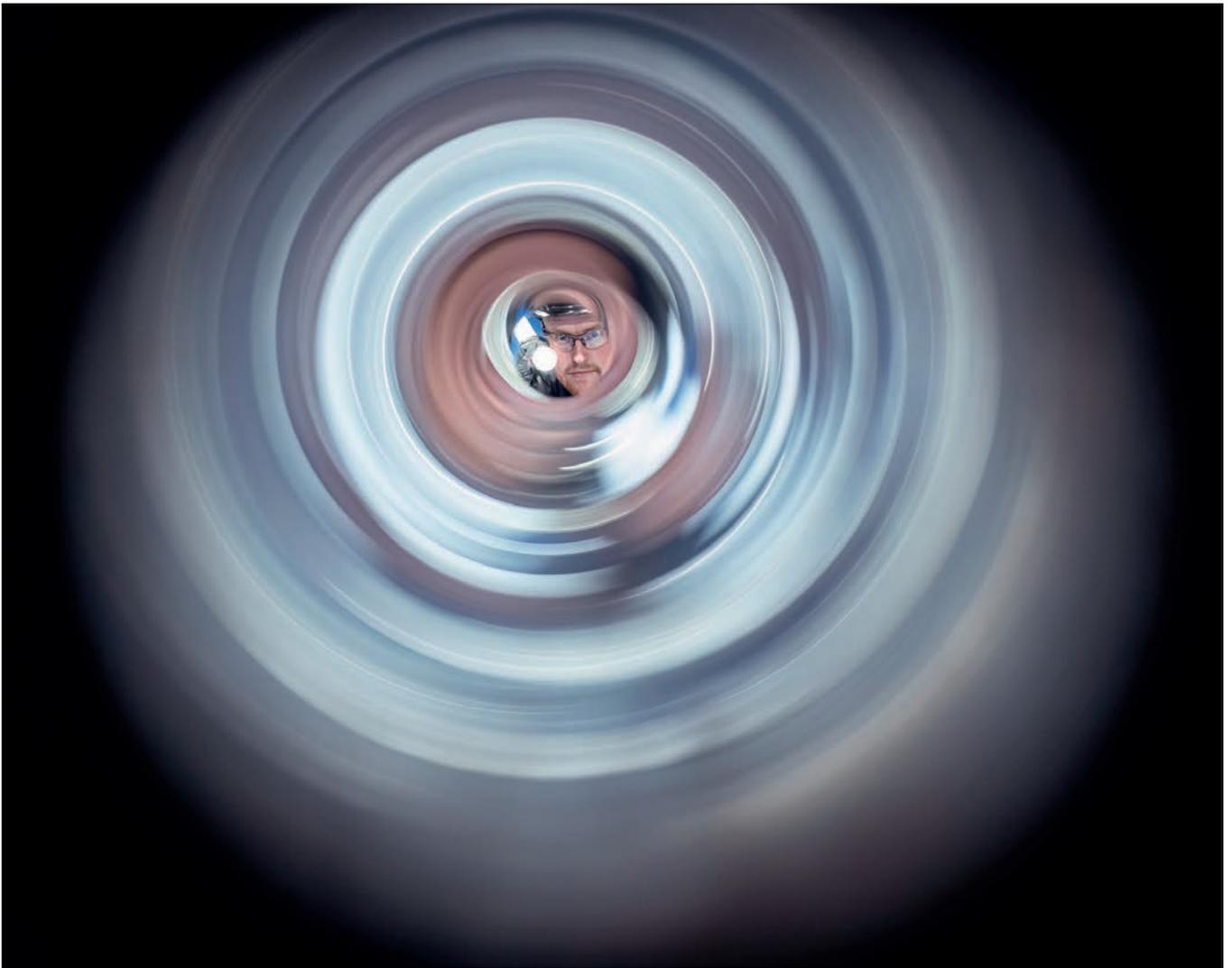
It takes 3 kilograms of gunpowder to set off First Light Fusion's two-stage big friendly gun to blast a projectile at a target that contains fusion fuel. The company first achieved fusion in 2021 © First Light Fusion
