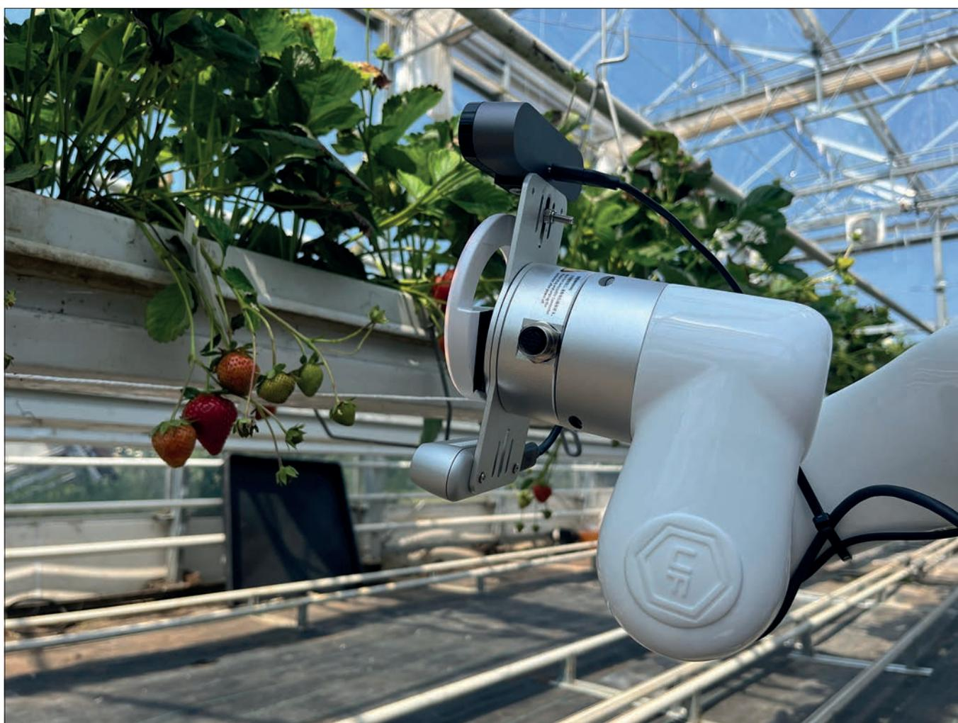
Robots are increasingly being used for autonomous monitoring and inspection. Here, the robot is checking the ripeness of strawberries but the same set up can monitor for other things such as pest and diseases © Warwick Agri-Tech at WMG, University of Warwick
