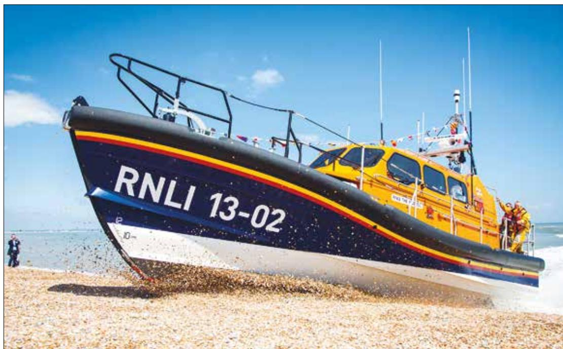
Being powered by water jets enables the Shannon to launch itself out of the sea and onto the beach easily without risking damage to a traditional rudder and screw propulsion system. The outer layer of the hull is also thicker than needed so that it is resistant to shocks and scratches © RNLI
