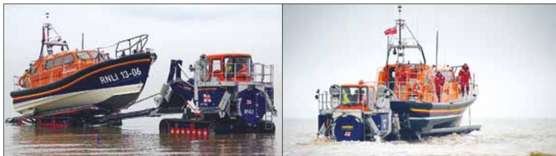
The Shannon can be recovered from the sea by the launch and recovery tractor. The boat sits on a 'slewing ring' that can be turned 180 degrees to relaunch the boat almost immediately © RNLI
