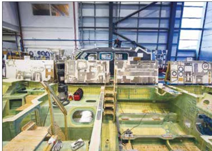
The entire construction of the Shannon takes place at the Poole All-Weather Lifeboat Centre. Each composite is created separately and joined together in a process that operates like a production line. A boat is completed every two months, resulting in six new boats a year © RNLI
