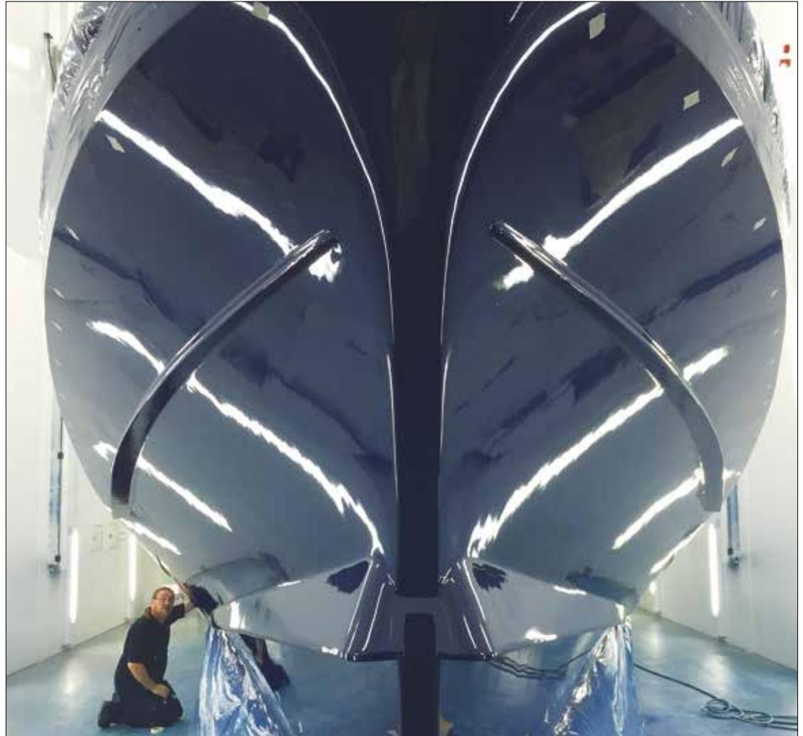
The Shannon's hull was completely redesigned, after a competitive tendering and testing process. The shape and angle of the sides of the new hull reduce broaching when the boat is travelling in the same direction as the swell © RNLI
