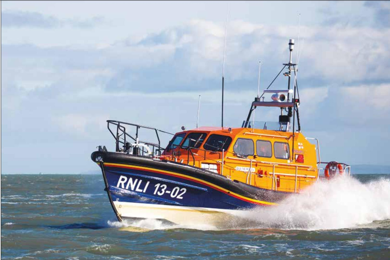
The Shannon lifeboat's hull is narrow at the bow, wider in the aft section and steeper in the mid region. This a shape that provides good stability and minimises slamming, which can put high stress on a vessel © Mike Lavis
