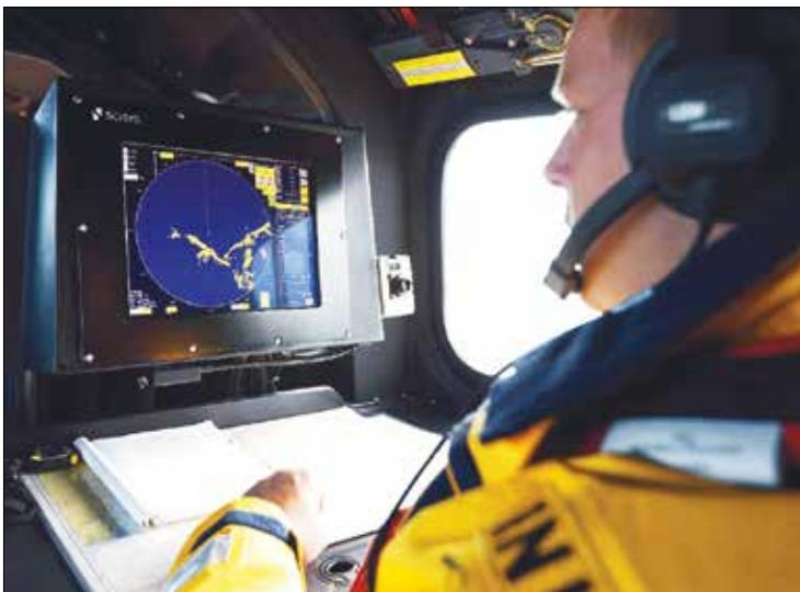
The systems and information management system provides access to the vessel's intercom and other communications, displays navigational information such as radar, charts, depth and speed, and data about the performance of the engines and other machinery © Nigel Millard
