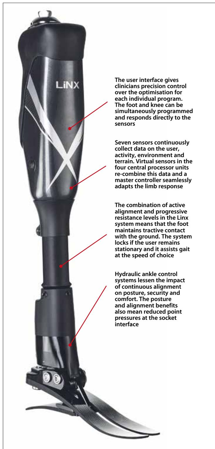
The user interface gives clinicians precision control over the optimisation for each individual program. The foot and knee can be simultaneously programmed and responds directly to the sensors
