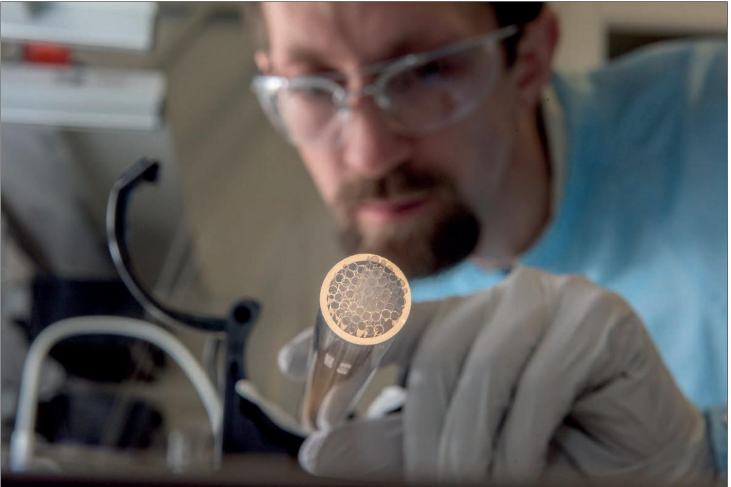
A cane preform being prepared in the Optoelectronics Research Centre lab in the University of Southampton's £120 million cleanroom complex
