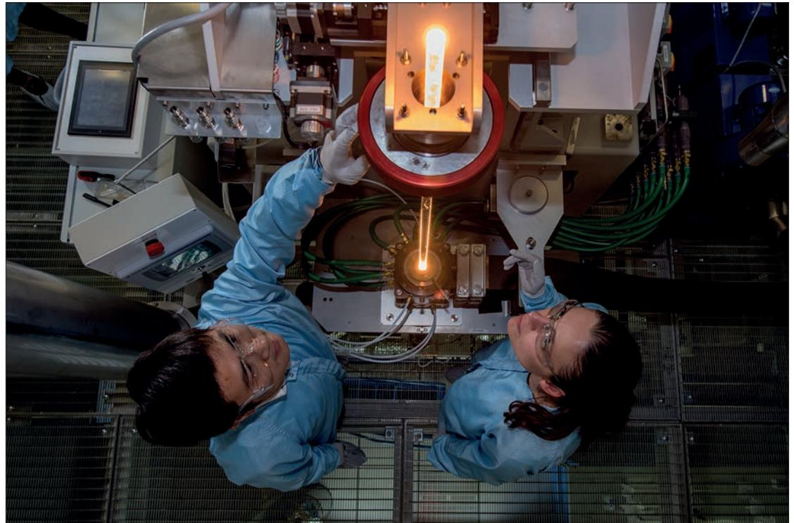
A fibre preform being fed into the furnace at the top of the fibre optic draw down at the Optoelectronics Research Centre fibre optic draw tower
