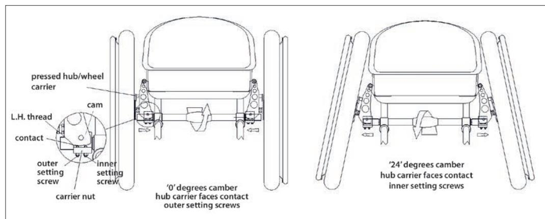
Diagrams show the mechanism that enables users to reangle their wheelchair's wheel © Trekinetic
