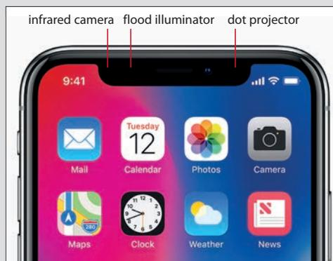
**The iPhone X's 3D facial recognition technology projects over 30,000 dots onto a user's face to map their features and uses the information to unlock the phone in the future. The dots are invisible to the human eye but can be seen through an infrared camera, which captures the image and sends the data for confirmation. The flood illuminator is an invisible infrared light that identifies facial features even when it's dark**
