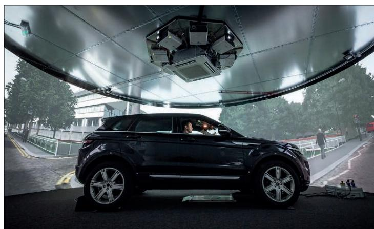
**The 360° driving simulator allows testing of smart and connected vehicles in a safe, controlled immersive environment**
