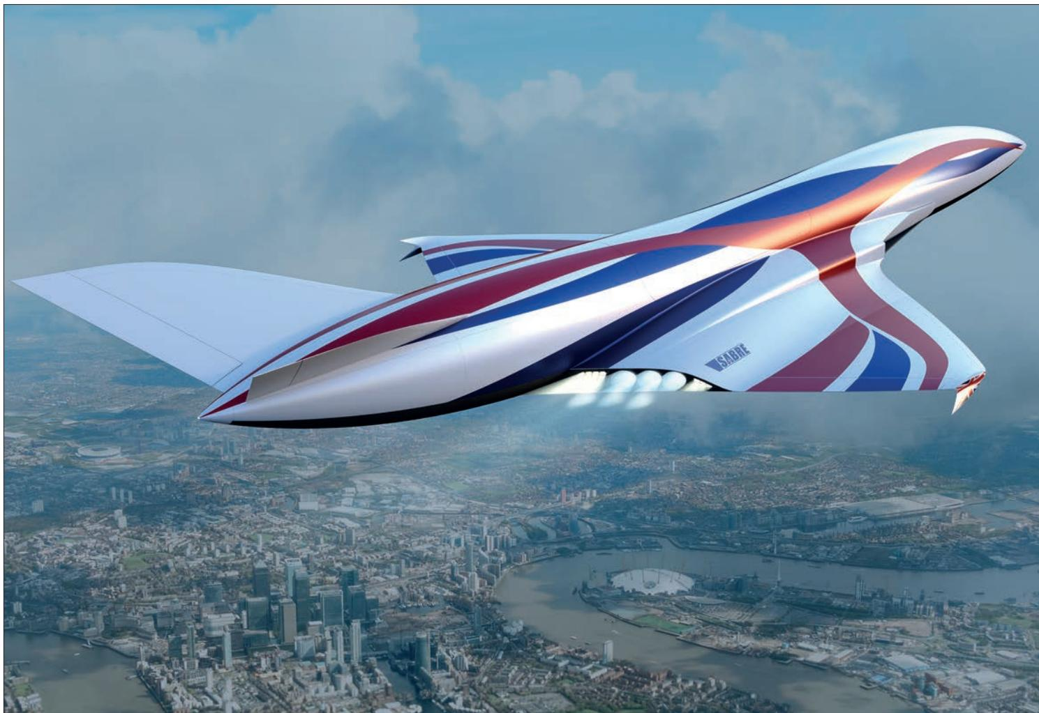
The SABRE engine could power flights across the world at five times the speed of sound © Reaction Engines
