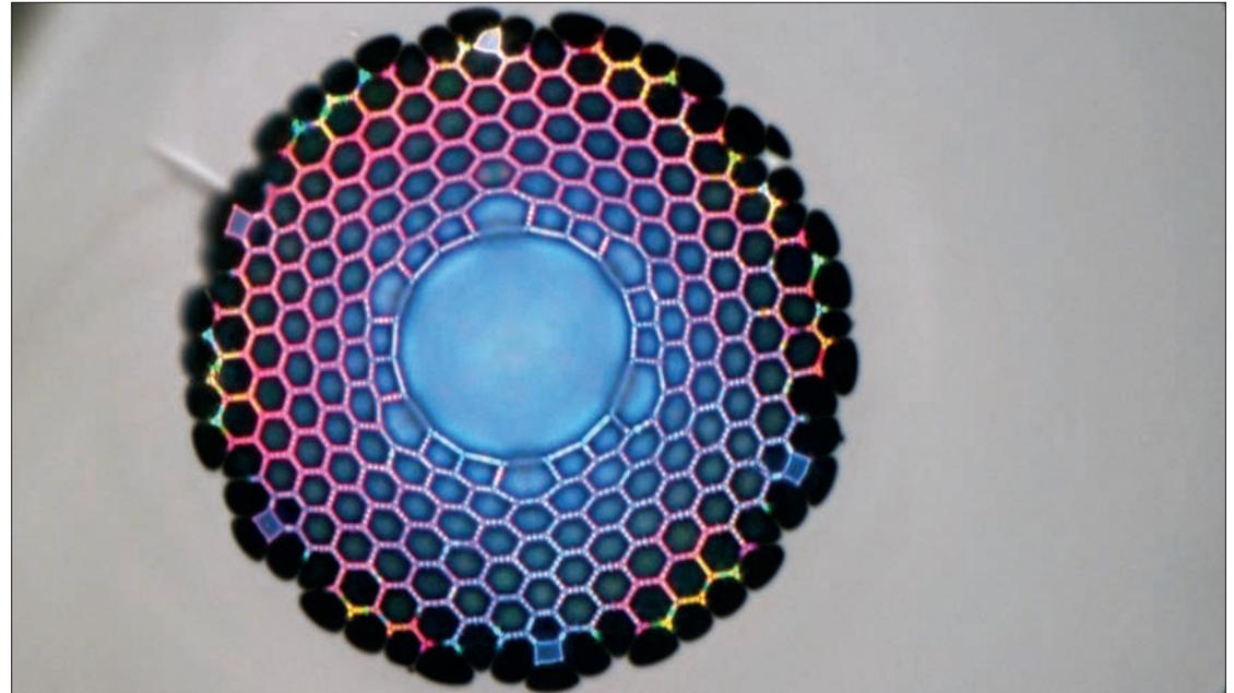
**A photonic bandgap type hollow core fibre with a large central core and honeycombed cladding**
