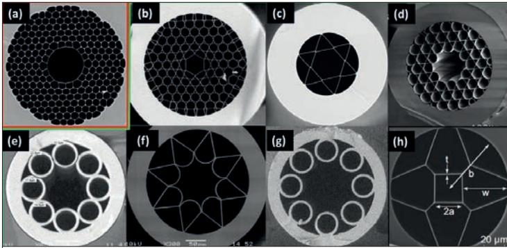
The range of hollow core fibre types available: a) Photonic band gap fibre; b to h) Various anti-resonant fibre designs (reproduced from Poletti F (2014) 'Nested anti-resonant nodeless hollow core fiber', *Opt. Express* 22, 23807-23828)
