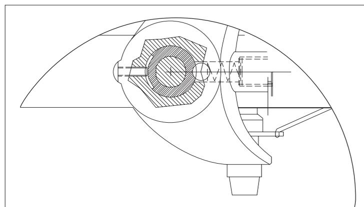
When going forward, a ballbearing sits in a detent (a catch that prevents motion until released), which locks the wheel into a straight position. When enough lateral force is applied, the wheel can twist away from that detent position and steer. The twisting force necessary will be different for each person so an especially designed adjustable spring was made and the detent shaped to control the way the ball moves away from its locked position
