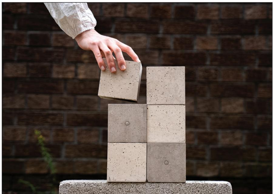
**Material Evolution’s low-carbon cement uses an alkali fusion process. This involves reacting an alkaline solution with slag from blast furnaces (or materials with similar properties). The mixture hardens into a powder, just like Portland cement**
