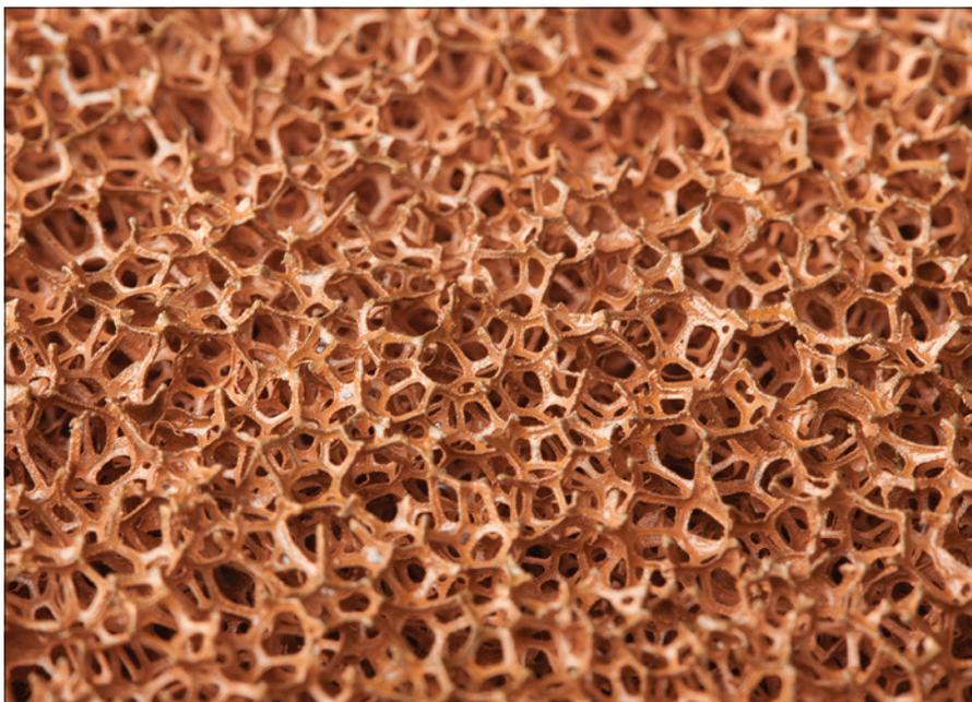
**To store energy using phase change material, engineers incorporate them into porous matrix materials, such as metal foams** © Shutterstock
