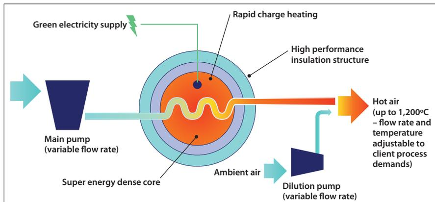
**Edinburgh firm Exergy3 has developed a high-temperature sensible heat storage system. Inside what looks like a standard shipping container, green electricity supplies a rapid charge heating system, which keeps ceramic bricks at 1,200°C in a cubic chamber. The chamber is surrounded by concentric layers of heat exchangers and insulation. Air pumped through the core is heated up to 1,200°C and used to drive industrial processes**
