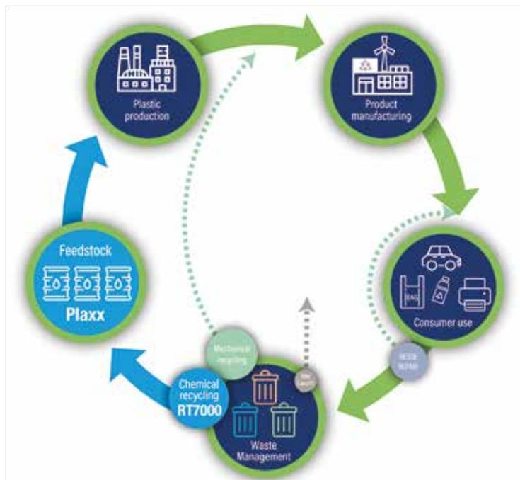
Keeping plastics in the circular economy: chemical recycling enables waste plastics to be converted to oil for making virgin-quality polymers, suitable for all applications, including food-grade plastics © Recycling Technologies
