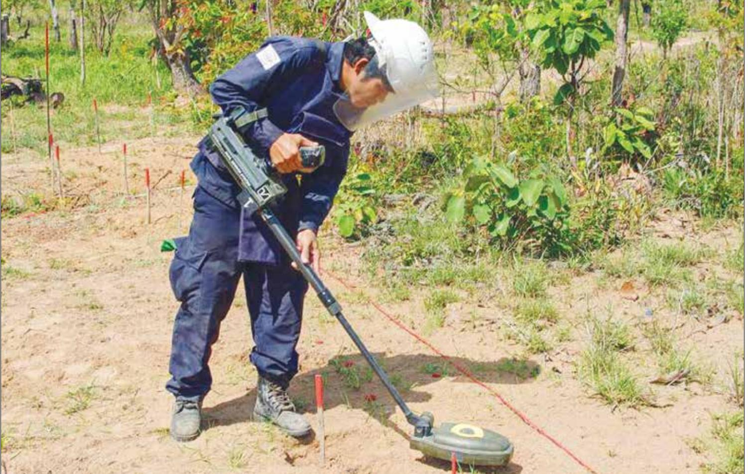
Humanitarian deminers in Cambodia evaluated a dual-sensor detector, which combines a metal detector and ground-penetrating radar, to search for landmines. The evaluation covered more than 600,000 square metres of land and removed over 5,600 landmines © The HALO Trust
