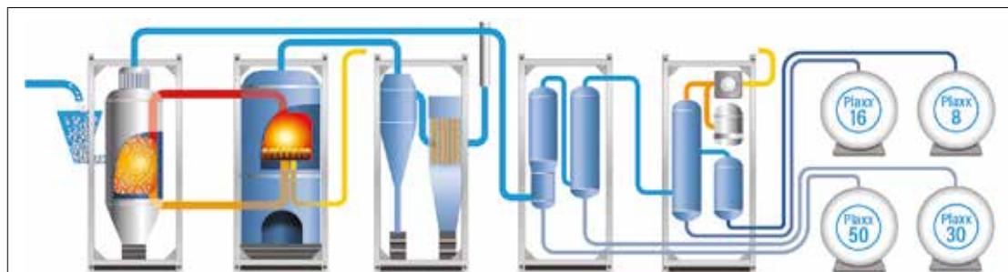
**The pyrolysis process, also known as 'thermal cracking', uses heat in the absence of oxygen to break down plastics**
