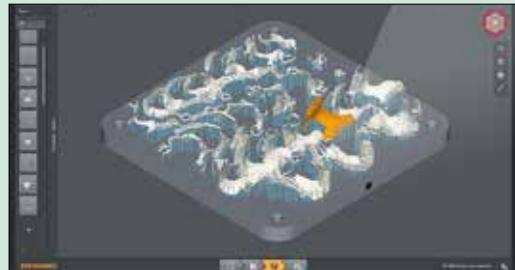
The design data is then prepared for build. This is where the build orientation is determined, ID tags and build supports are added to each part and, finally, the parts are nested.
