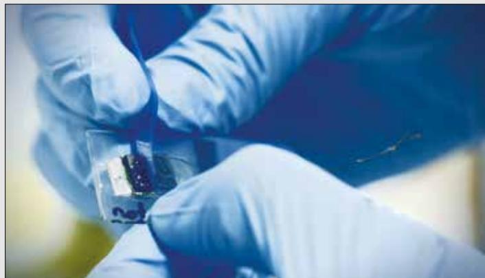
**A variety of methods exist for producing graphene on a mass scale, but Scotch Tape remains a favourite in labs across the world**
