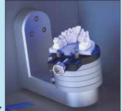
A lab scanner digitises the model, often using structured light scanning.
