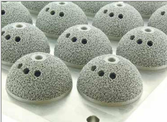
**Recent advances in AM include the development of load-bearing lattice structures for orthopaedic implants. By incorporating a lattice, implants can provide a scaffold structure for new bone tissue to grow into, with the spacing and strut thickness of the lattice optimised to match the stiffness of surrounding bone. The lattice, with its ‘pseudo-random’ internal structure, would be near impossible to manufacture in any other way than AM © Renishaw**
