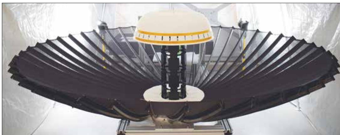
Oxford Space Systems' deployable structures, such as this wrapped-rib antenna, use novel design techniques based on origami so that they can be folded and stowed more efficiently © Oxford Space Systems
