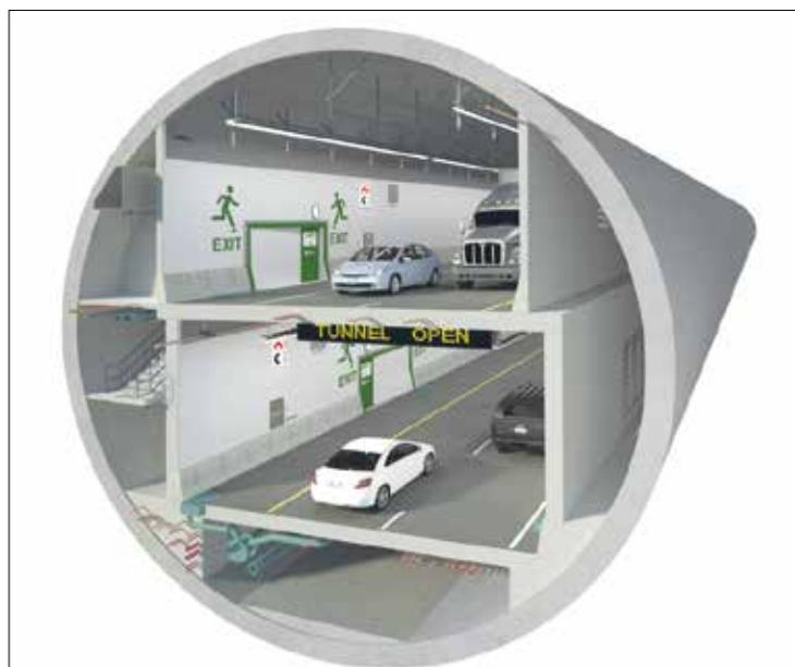
A computer-generated image depicts a cross-section of the Alaskan Way tunnel, showing four lanes of highway with two at the top and two at the bottom © Washington State Department of Transportation
