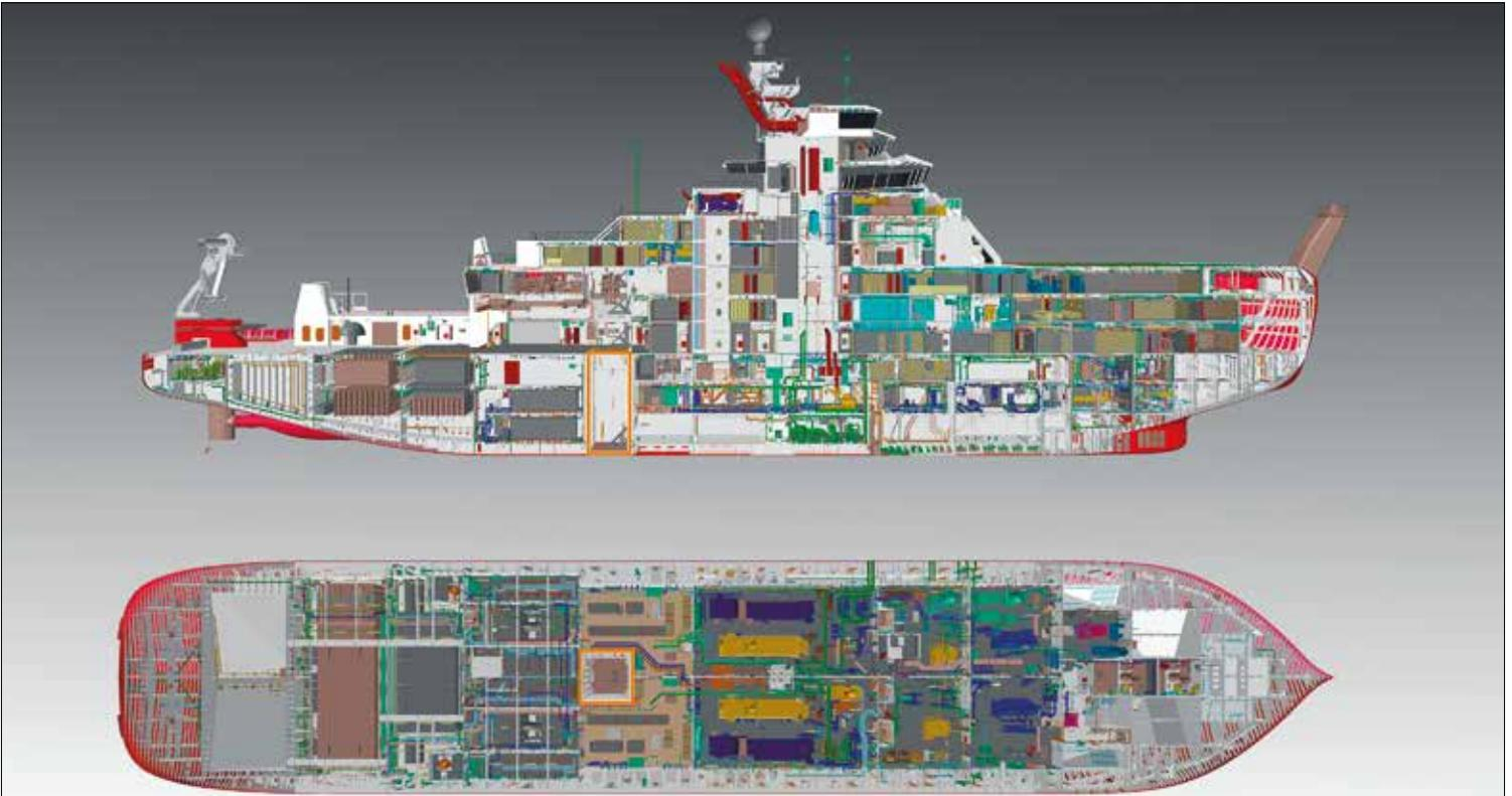
The RRS *Sir David Attenborough* is the first British polar research ship to have a moon pool – its location on the ship is indicated by the orange coloured squares on the image above. A watertight, hydraulically-operated single leaf door secures the moon pool, and opens to leave a four metre by four metre clear space through to the bottom of the ship. The trolley arrangement that is used to guide equipment into the ocean can be seen just above the coloured box on the top image © Rolls-Royce
