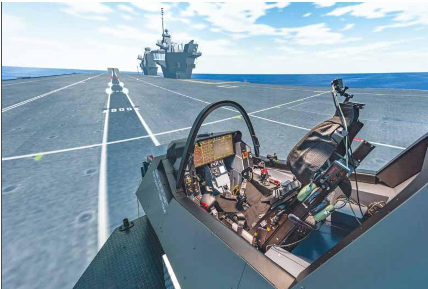
**The fully immersive simulator has a cockpit moved by an electric motion platform. Highly specialised engineering data was fed into the simulator to replicate the disturbances that an aircraft would experience, meaning that when a pilot lands an F-35 in the simulator, they feel the motions that they would feel in real life** © BAE Systems
