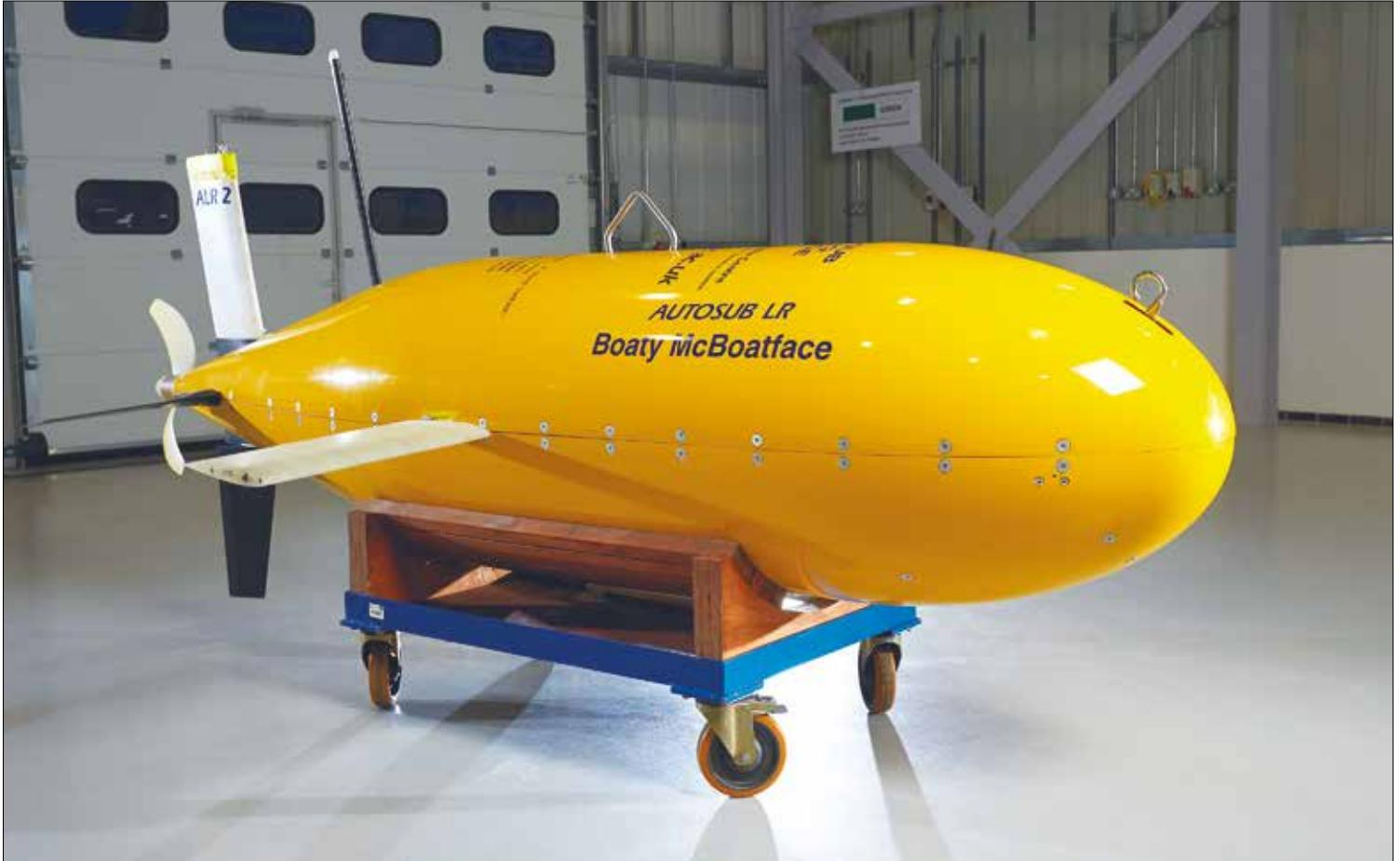
**Boaty McBoatface is one of several autonomous unmanned vehicles onboard the RRS Sir David Attenborough. Robotic submarines and marine gliders will collect data on ocean conditions and marine biology and deliver it to scientists working in the ship's onboard laboratories** © National Oceanography Centre
