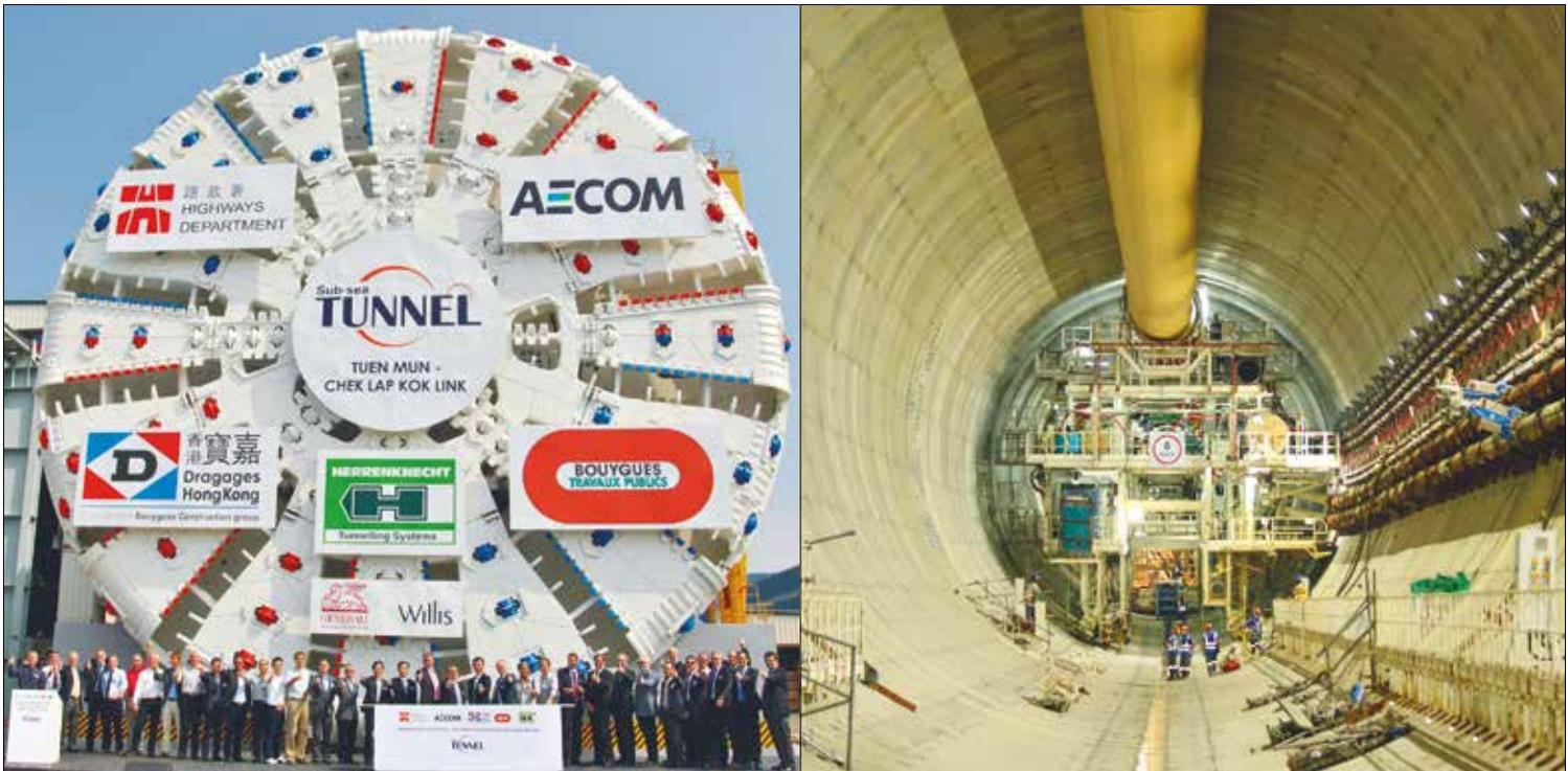
Left: The world's largest ever tunnel boring machine, the 17.6-metre-diameter slurry tunnelling machine prior to its use to drive a part of the Chep Lak Kok to Tuen Mun subsea tunnel in Hong Kong; right: The smaller 14-metre-diameter tunnel boring machine driving one of the twin tunnels for the Hong Kong tunnel
