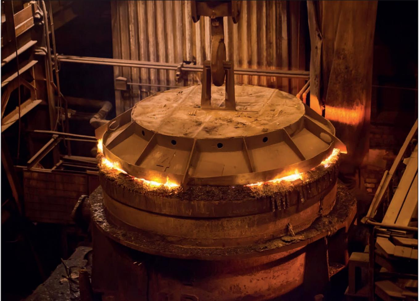
**An electric arc furnace. Its characteristic domed roof is closed over the bowl-shaped hearth. Electrodes protruding from the roof are melting scrap steel inside** © Shutterstock
