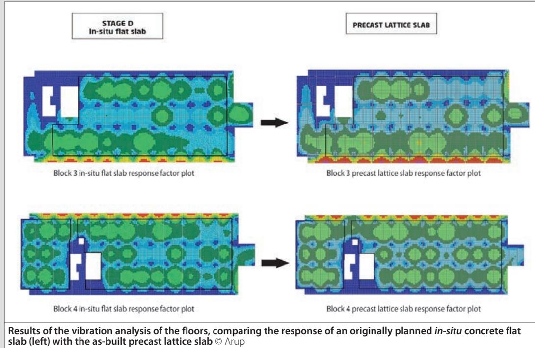
The Francis Crick Institute has been constructed with a remarkably high resistance to vibration, but the NMR and MRI scanners in the basement required an additional level of protection.
