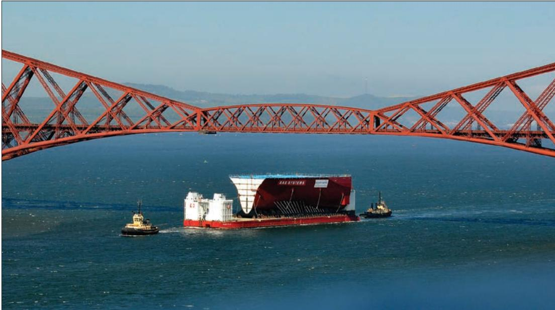
Many of the larger blocks, which have been fitted together like a jigsaw to build each vessel, weighed in excess of 11,000 tonnes and required the world's biggest submersible barge to transport them around the UK to Rosyth, Fife
