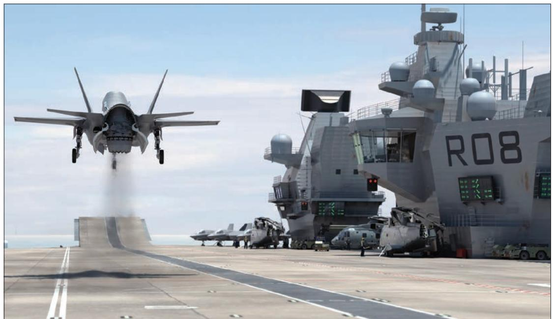
**Each vessel will carry 36 of the new F-35B short take-off and vertical landing jets. The exhaust jet produced by these aircraft has meant engineers have had to develop an entirely new deck coating to protect it from the extreme heat**
