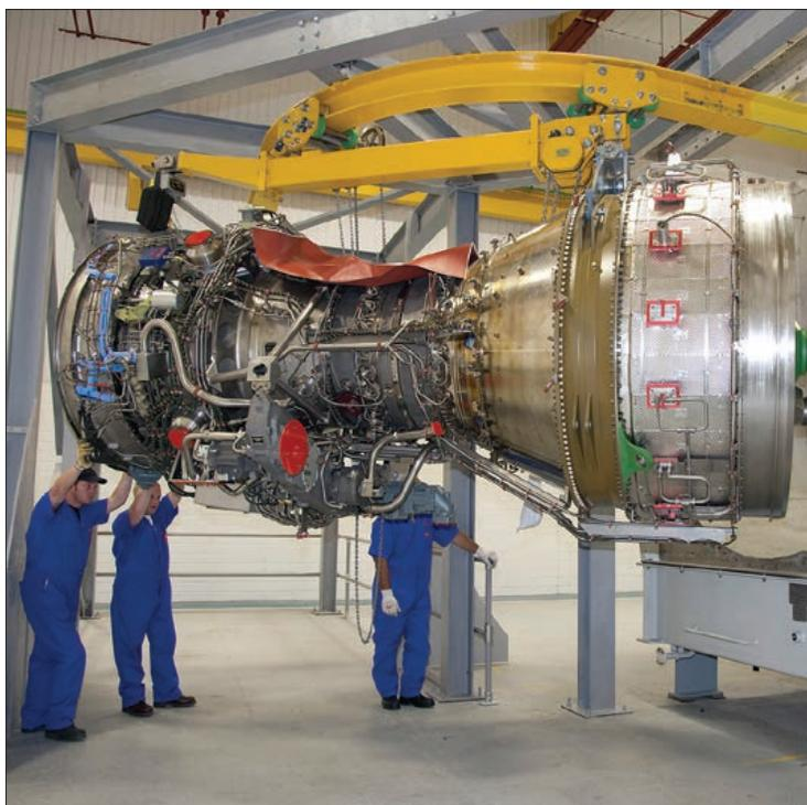
Each of the aircraft carriers is powered by two Rolls-Royce MT30 gas turbines and four diesel generators, which together produce a combined output of 110 MW. One of the MT30 gas turbines is pictured above © Rolls-Royce
