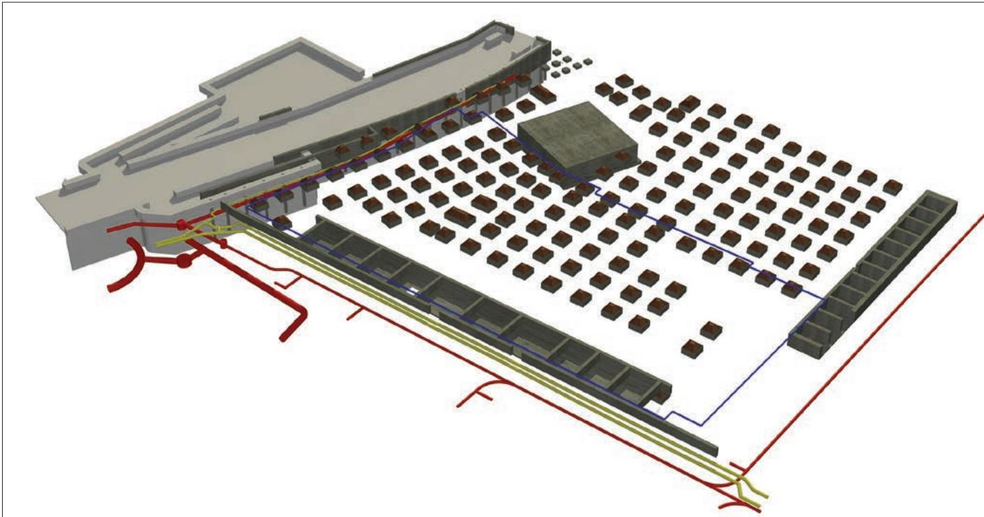
The site was constrained on all sides, with the buried structure of St Pancras Thameslink platforms to the east (left of picture), two Victorian cast-iron gas mains to the north, old brick-arch sewers to the north and west, and the British Library's buried pumping station to the south. The site itself was once a railway goods depot, and was underlain by a grid of brick footings on mass concrete which had to be removed © AKT II
