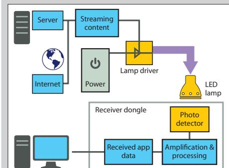
Data is streamed via an LED lamp with signal-processing technology
