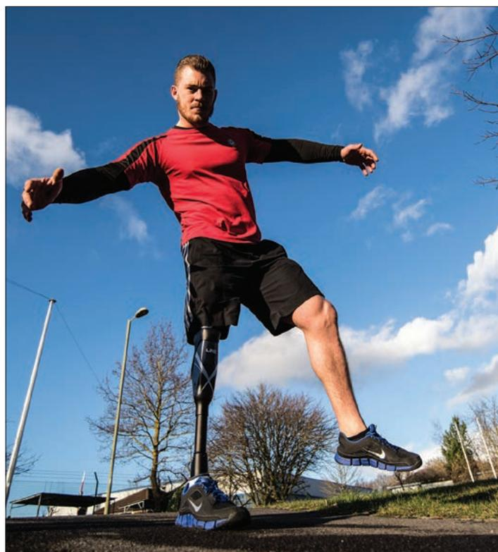
The Linx limb system's sensors act like human nerves to inform the prosthetic's response so that users can walk, balance and be supported on all types of terrain © Blatchford Group
