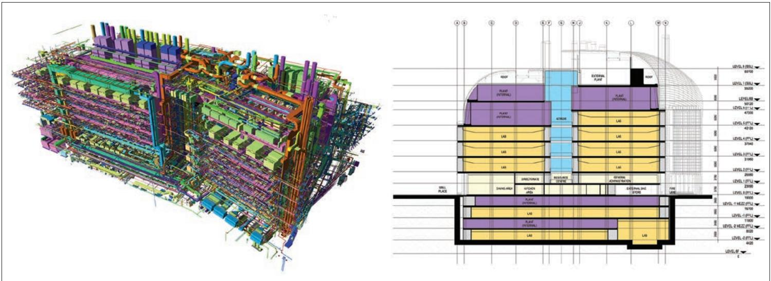
A three-dimensional building information model of the complex and extensive engineering services, so that the building resembles a massive industrial plant with some working space sandwiched in between. As the cross-section through the building shows, two of the four basement levels and three of the eight above-ground levels are mainly filled with services © Arup
