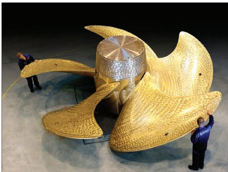
Two 33-tonne propellers, one of which is pictured above, will drive HMS Queen Elizabeth and HMS Prince of Wales through the water. They have been designed so their pitch can be modified to aid propulsion through the water © Rolls-Royce
