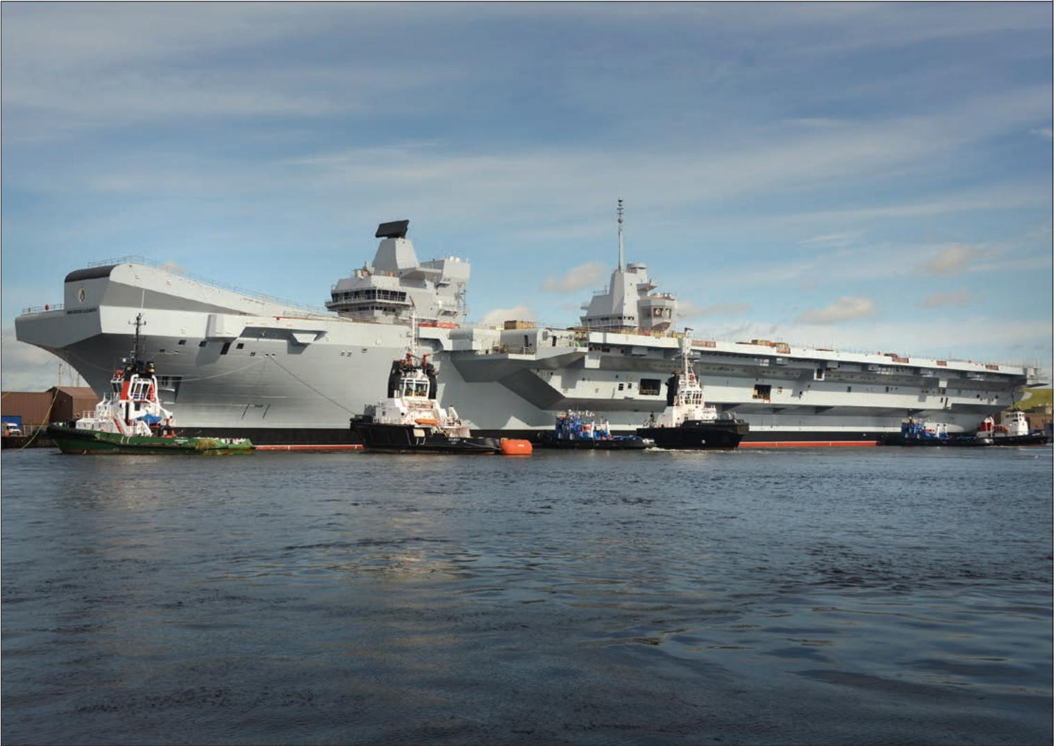
From keel to masthead, the HMS Queen Elizabeth towers 56 m in height and the overhanging hull supports a flight deck covering 4.5 acres © Aircraft Carrier Alliance
