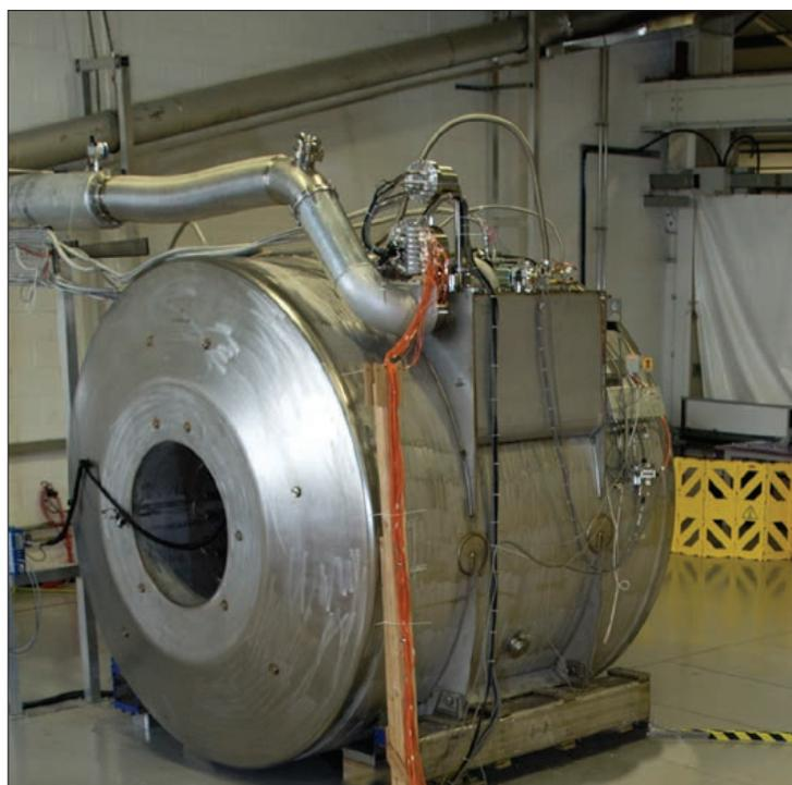
The 7 Tesla magnet has now been incorporated into the MAGNETOM Terra system, which will offer clinicians and researchers access to the best of MRI imaging © Siemens Magnet Technology
