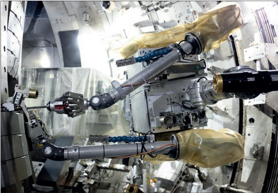
**The Joint European Torus fusion facility in Oxfordshire has recently upgraded its remote handling robots to help it with decommissioning. MASCOT, pictured, has haptic feedback that allows the operator to feel every action from carrying a new component to tightening a bolt** © UK Atomic Energy Authority
