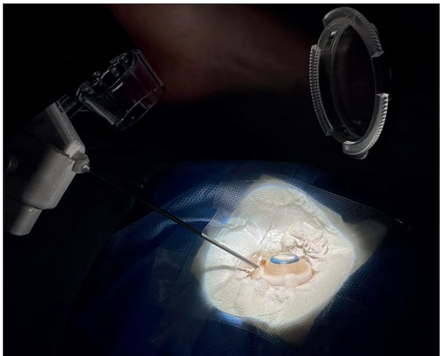
Close up of the experimental setup illustrated in the next figure. A phantom eye with dimensions and appearance similar to a human eye is used for evaluation. The surgical tool is approaching the eye to be inserted through a trocar (orange insert)
