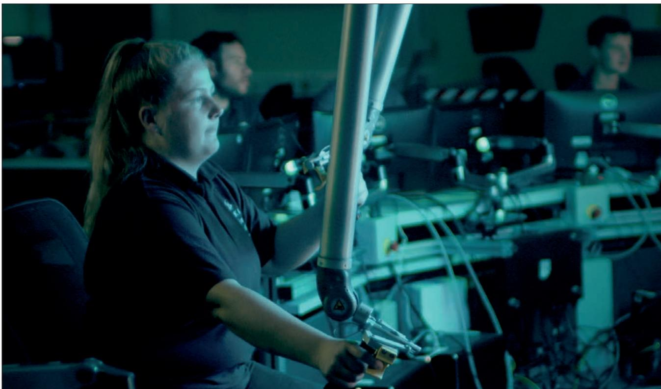
**Charlotte Wilkes, an apprentice mechanical design engineer at the UKAEA, controlling the remote manipulation system at JET**
