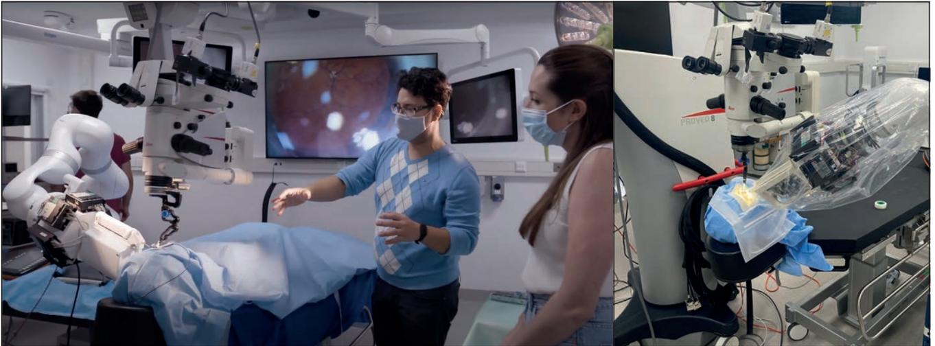
**Left: The developed robotic system, showcased within the mock operating room of the Department of Surgical and Interventional Engineering at King's College London. Right: Illustration of potential system draping, so that it can enter the sterile zone of an operating room** © Left image courtesy of China Global TV Network
